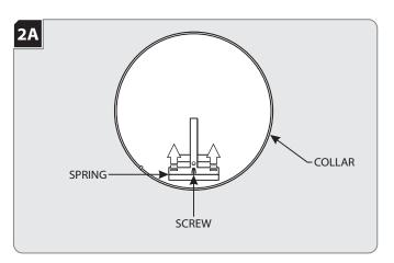
Release the spring by removing the screw.
